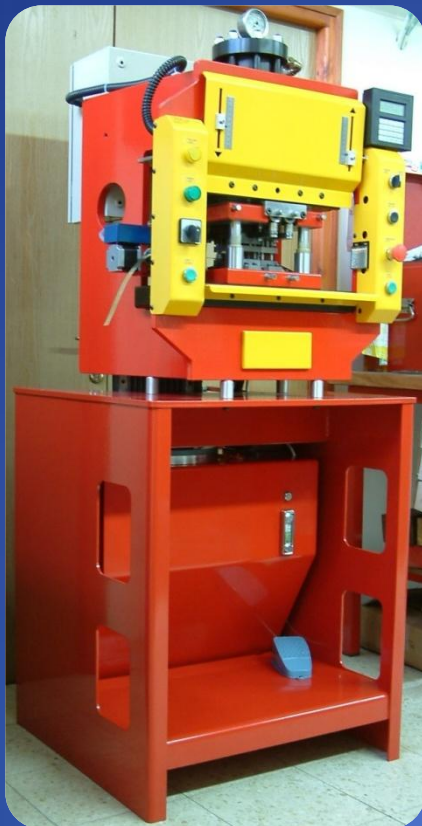
Proment 15 Ton press including bench (W=763mm, D=1000mm. H=1592mm.)
