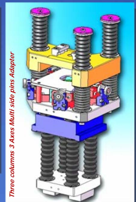
*Three columns 3 Axes Multi side pins Adapter*
